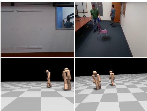
Figure 9: Through wall example. The top left image represents the view of the radio, the top right image shows the view inside the room. Bottom row shows the detected skeletons in corresponding views.
