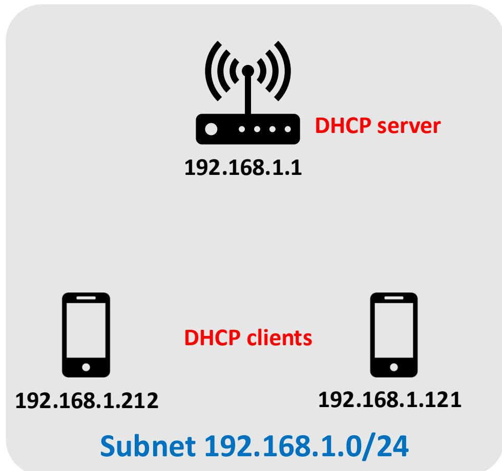
Typically, DHCP server will be co-located in router, serving all subnets to which router is attached
