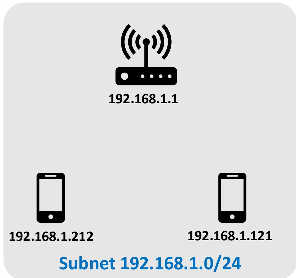
**goal:** host *dynamically* obtains IP address from network server when it “joins” network
