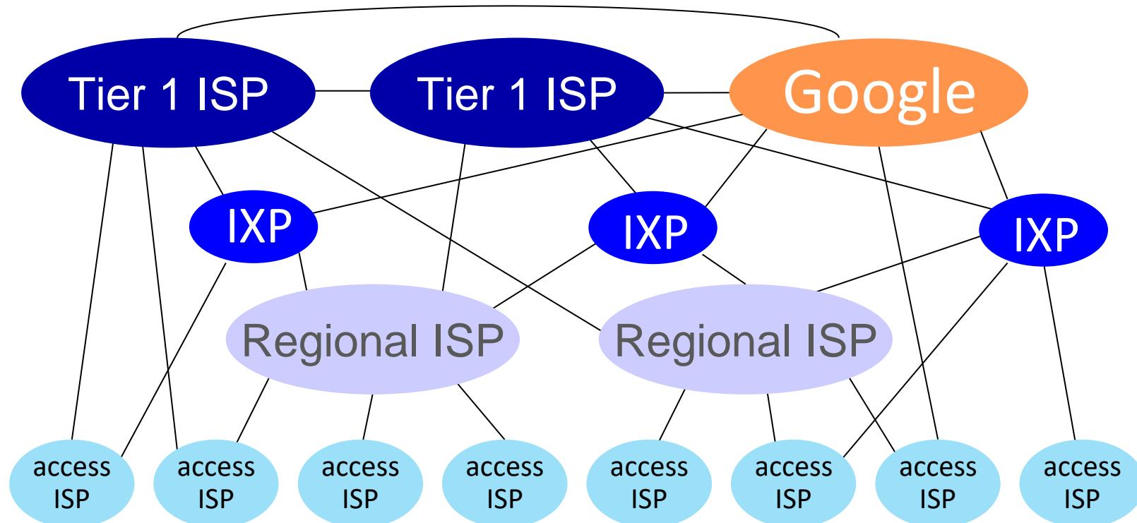
At “center”: small # of large but well-connected networks
