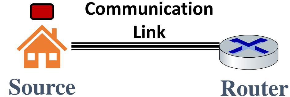
**Step 1: Transmit the packets into the link**
