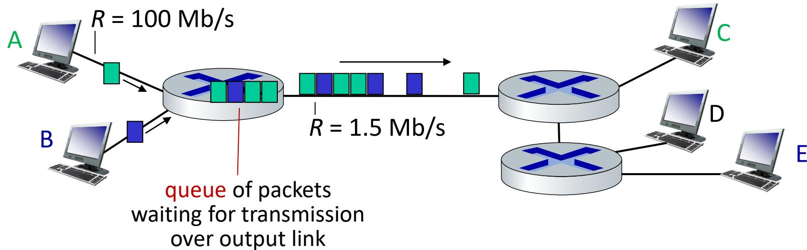
*Packet queuing and loss:* if arrival rate (in bps) to link exceeds transmission rate (bps) of link for some period of time:
